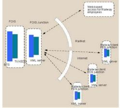
Figure 3 3-tier client server architecture
