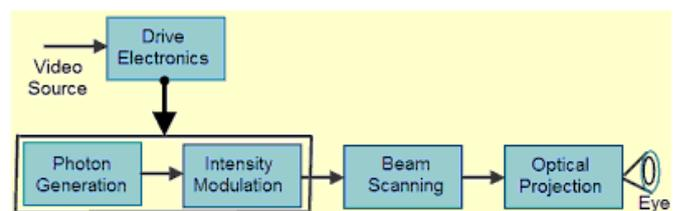
**Figure 2.2.1** Block Diagram of Retinal Display
