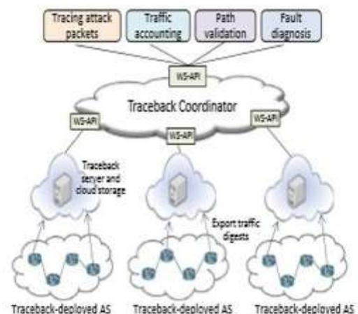
**Figure 1:** Architecture overview of cloud-based traceback.
