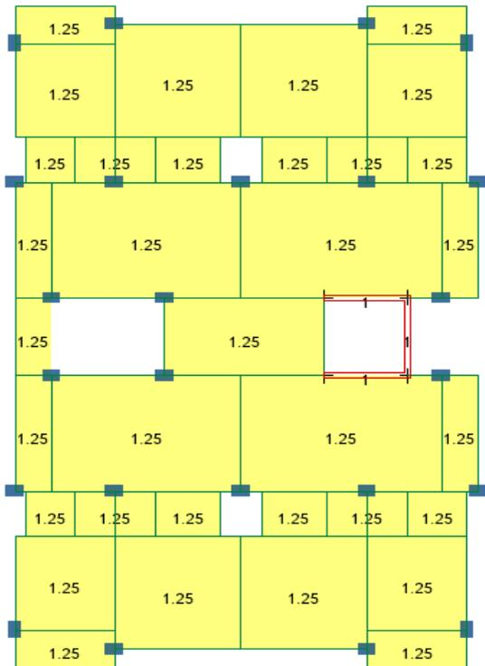
**Fig.4- Floor Finish Load (Super Dead)**
