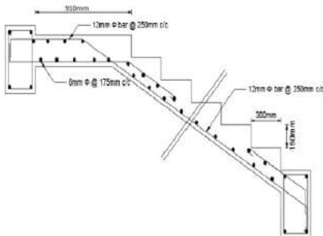
**Fig.18 Reinforcement detailing of staircase**
