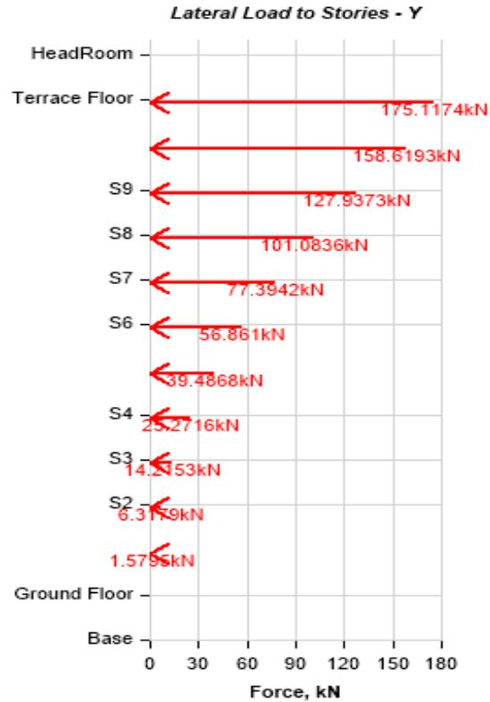
IS1893 2002 Auto Seismic Load Calculation
