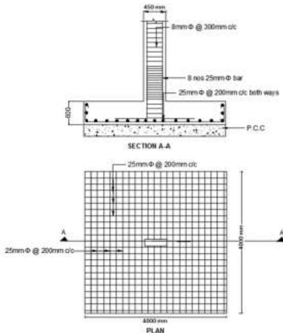
**Fig. 20 Reinforcement detail of footing**
