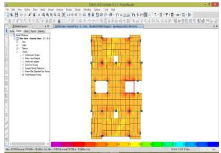
**Fig.10 Slab bending moment diagram**
