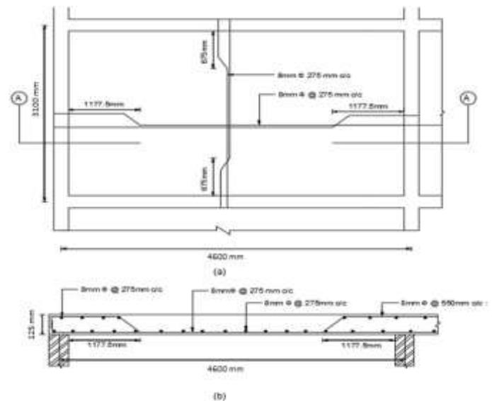
**Fig.16 Reinforcement detailing of two way slab**
