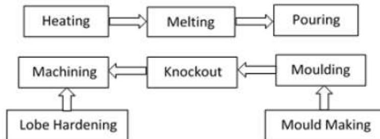
Figure 5. Casting process for manufacturing crankshaft
