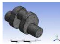
Figure 8. Meshed crankshaft in ANSYS
