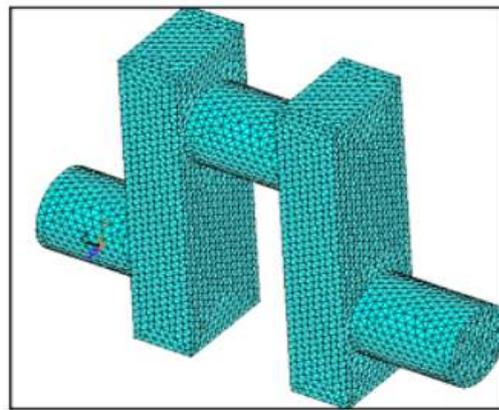
Figure 28. Meshed model in ANSYS
