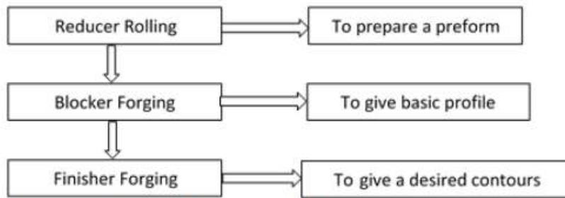
Figure 3. Stages in crankshaft forging
