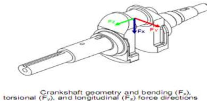
Figure 2. Forces acting on crankshaft
