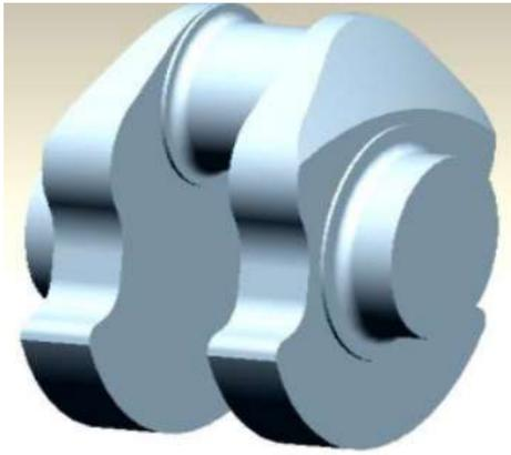
Figure 21. Model of crankthrow
