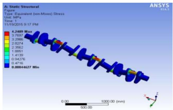
Figure 18. Von-Mises stress in Inconel X-750
