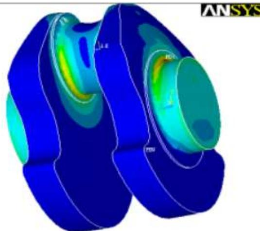
Figure 25. Total deformation in crankthrow    Figure 26. Von-Mises stress in crankthrow
