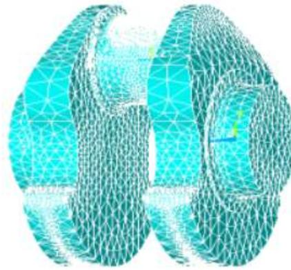
Figure 22. Meshed model of crankthrow
