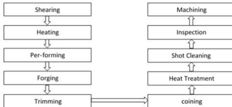
Figure 4. Forging process for manufacturing crankshaft
