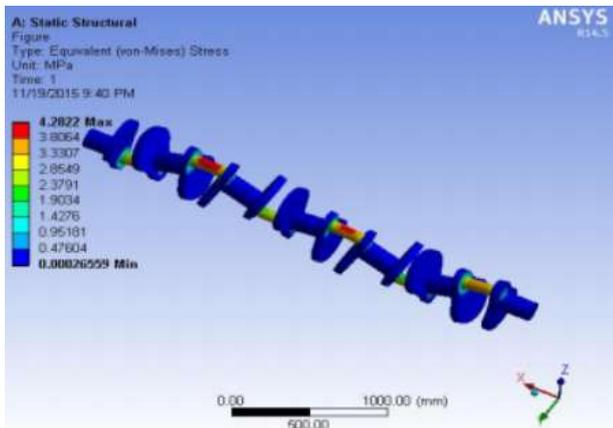
Figure 17. Von-Mises stress in steel
