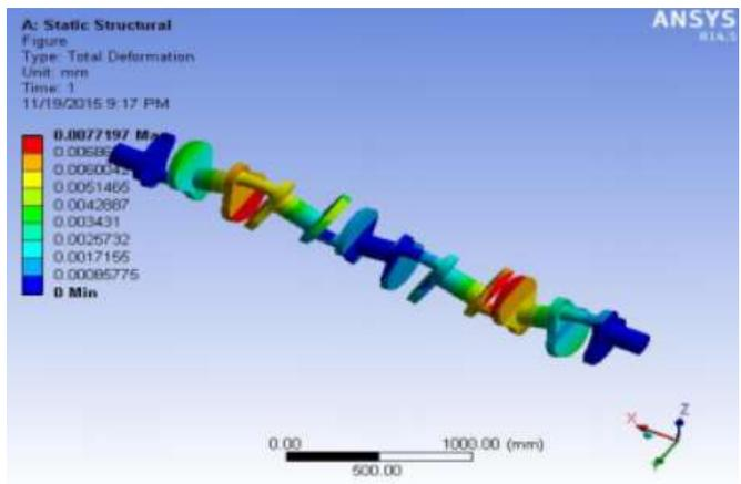
Figure 16. Total deformation in Inconel X-750
