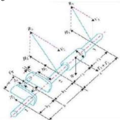
Figure 7. Forces acting on crankshaft when it is at the dead centre
