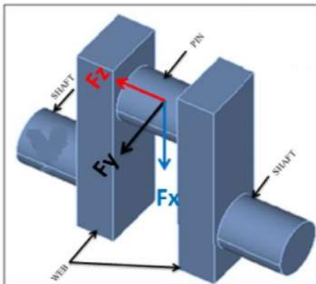
Figure 27. Crankshaft model in CATIA
