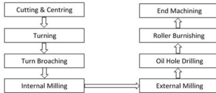
Figure 6. Machining process for manufacturing crankshaft
