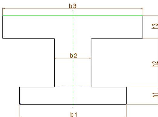
Figure 3: Axle I-section
