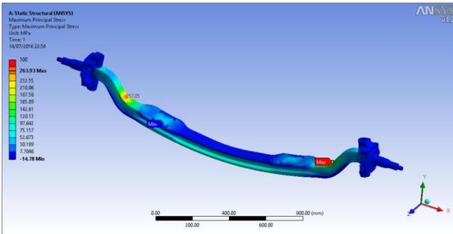
Figure 4: Analysis of Maximum Principle Stress
