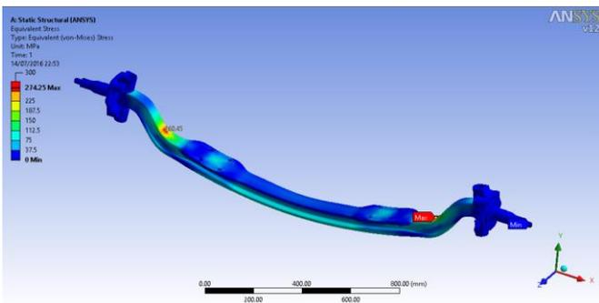
Figure 5: Analysis of equivalent (Von-mises) stress
