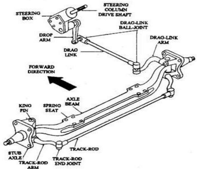
Figure 2: Front axle beam linkage assembly with Steering system
