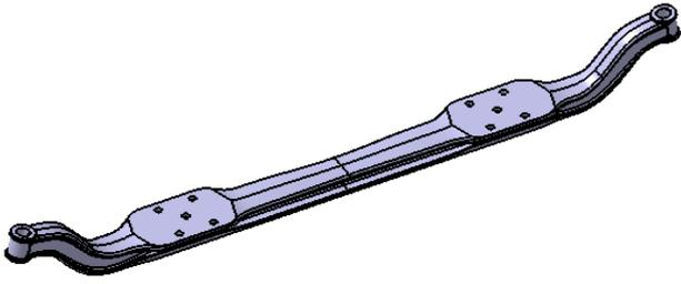
Figure 1: front axle beam
