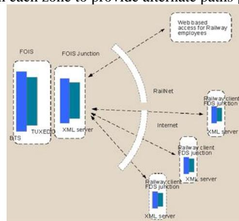
Figure 3 3-tier client server architecture
